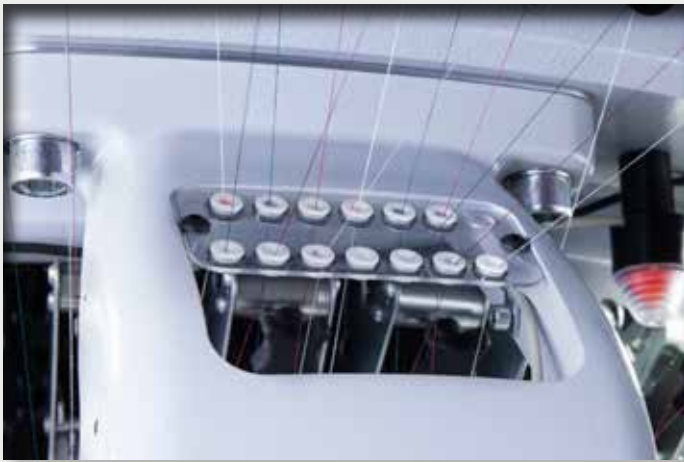
position of the elastomeric yarn in the yarn guide
